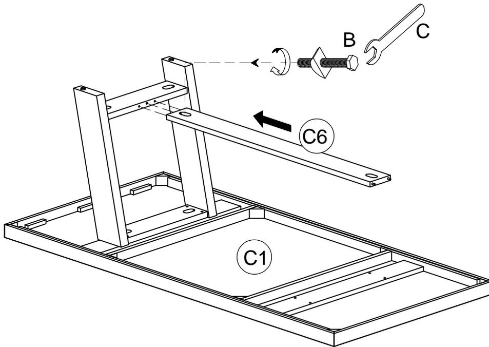
**STEP 4** Attach the Leg frame to the table top (C1) and Stretcher (C6), using bolt (A)(B).
