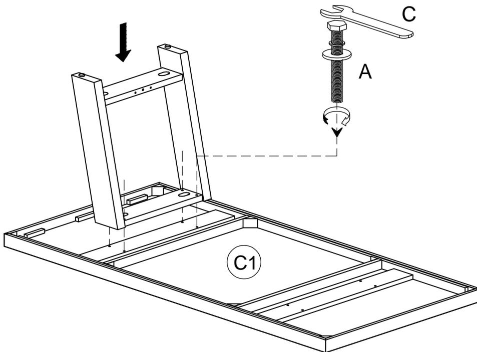
**STEP 3** Attach the Stretcher (C6) to the Leg frame, using bolt (B).
